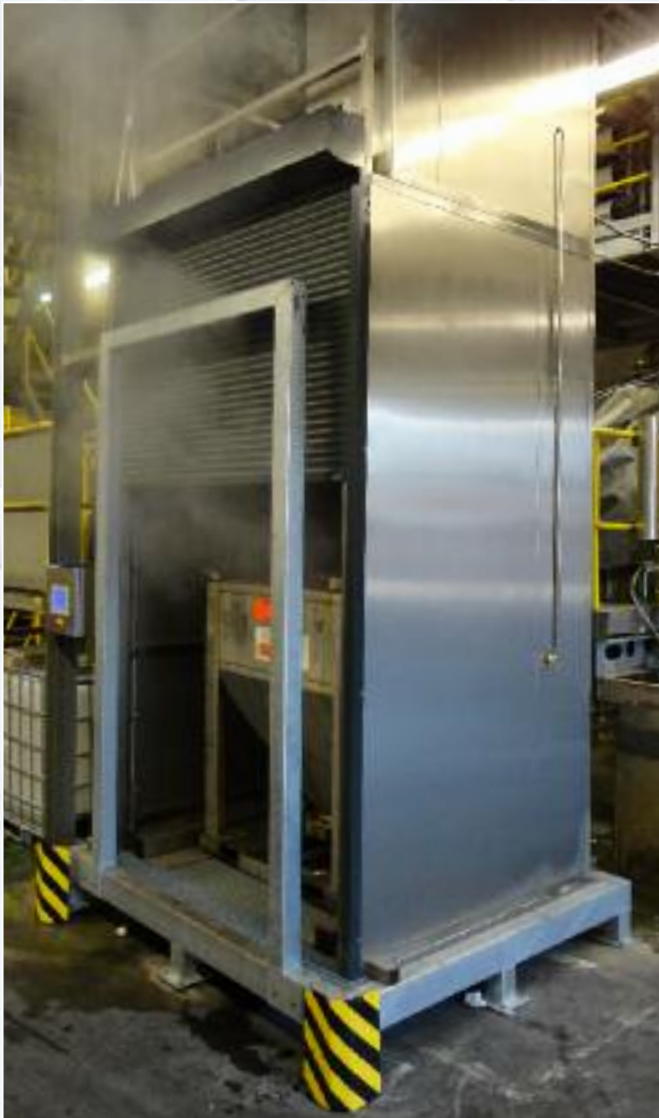
Full-automatic cleaning system for IBC containers.
