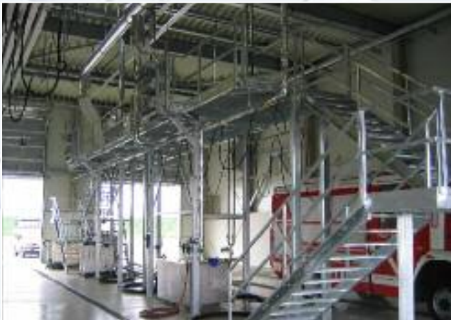
Tank cleaning station for interior cleaning in a cargo center.
