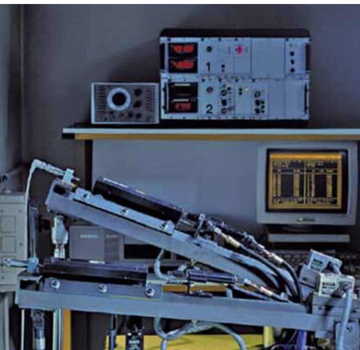
Very good demulsibility in the Schmidt-test: RENEPS slideway oils with ECOCOOL cutting fluids.
