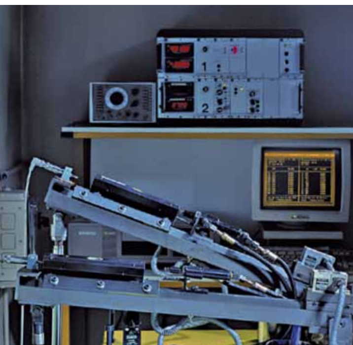
Very good demulsibility in the Schmidt-test: RENEPS slideway oils with ECOCOOL cutting fluids.
