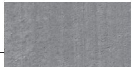
Scanning electron micrograph of the surface of a MoS 2 solid film lubricant layer after tribological loading by the friction partner – smoothing of the surface of the solid film lubricant.
